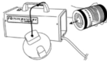
Insert open end of cartridge into back of machine, seating firmly against internal gasket. If substantial oil leakage is evident, do not use.
