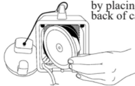
Retain lid for storage by placing against back of cartridge.
