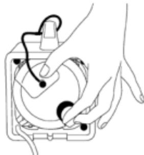
Install spring-loaded cover plate against cartridge lid & twist to lock into place.
