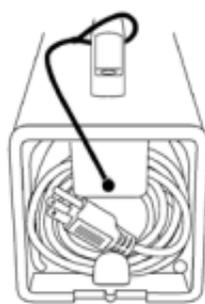
To operate, plug cord into power outlet. Always unplug Restorator before removing cartridge. The cord can be coiled for storage in the back of the rear cover plate.
