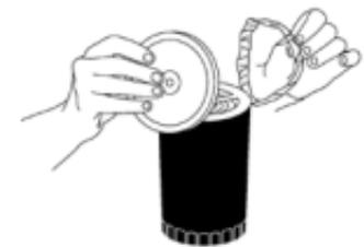
Turn off machine. Lift off cartridge lid & discard clear film liner. Cartridge life is rated at 270 hours.
