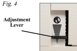
On unit's side is the air treatment adjustment lever. Move lever up to increase dry vapor output & down to decrease/turn off this function.
