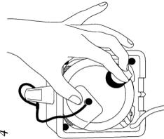
Install spring-loaded cover plate against cartridge lid & twist to lock into place.
