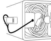
To operate, plug cord into power outlet. Always unplug Restorator before removing cartridge. The cord can be coiled for storage in the back of the rear cover plate.
