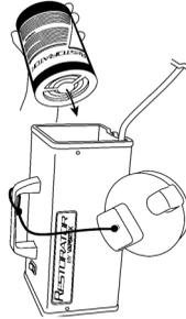
Insert open end of cartridge into back of machine, seating firmly against internal gasket. If substantial oil leakage is evident, do not use.
