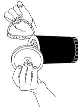
Turn off machine. Lift off cartridge lid & discard clear film liner. Cartridge life is rated at 270 hours.
